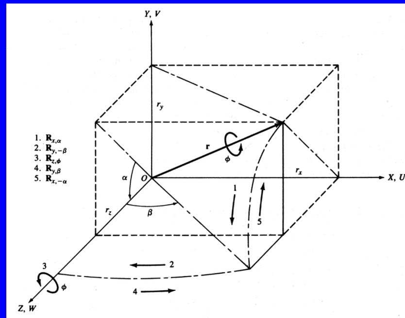
$$R_r(\phi) = R_x(-\alpha)R_Y(\beta)R_Z(\phi)R_Y(-\beta)R_x(\alpha)$$
