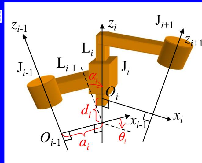
$$\tilde{p}_0 = {}^0T_1 T_2 \cdots {}^{n-1}T_n \quad \tilde{p}_n = {}^0T_n \tilde{p}_n$$
