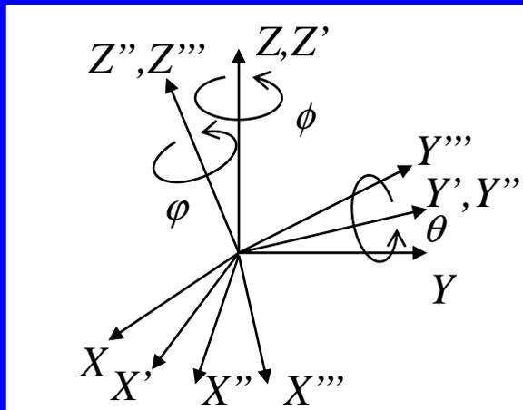
$$R(\phi, \theta, \varphi) = R_Z(\phi)R_Y(\theta)R_Z(\varphi)$$
