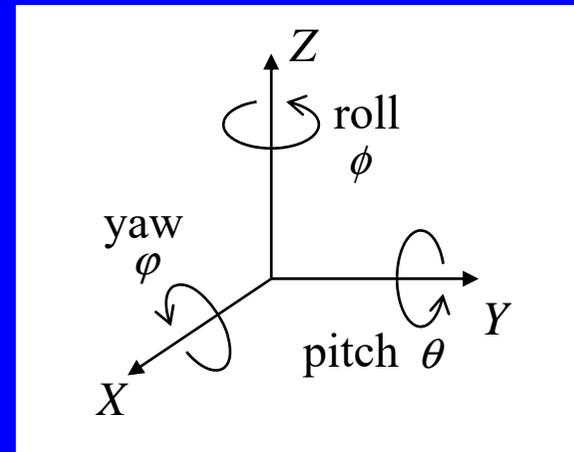
$$R(\phi, \theta, \varphi) = R_Z(\phi)R_Y(\theta)R_X(\varphi)$$
