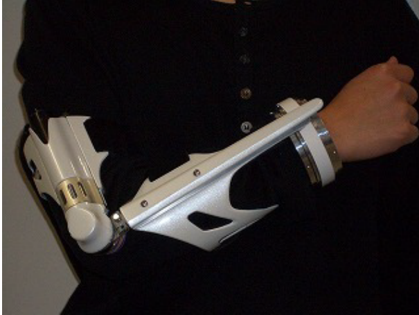
Fig. 1. Upper limb motion assist robot
